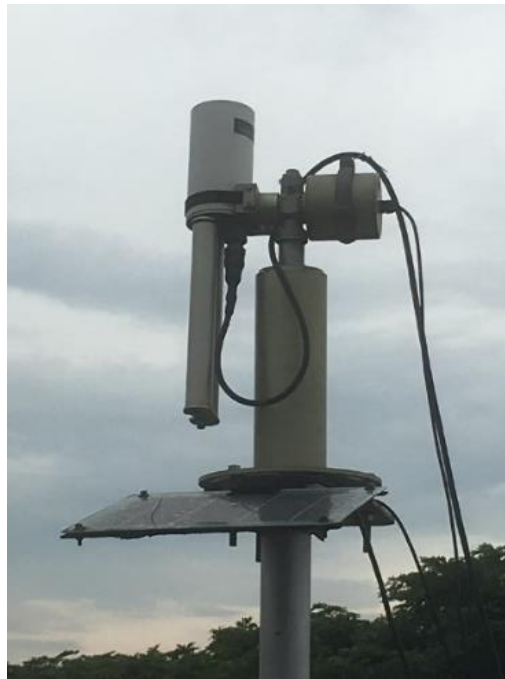
Figure 4. The AERONET sun photometer installed in Manila Observatory.
